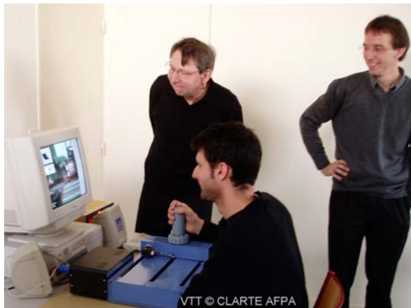
VTT project: a specific haptic interface developed by CLARTE with ESIEA
