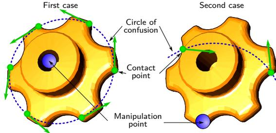
Figure 4: Two different configurations of manipulation: The manipulation point on the left is more likely to produce ambiguous vibratory renderings than the right one.
