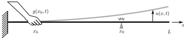
Figure 2: Cantilever vibrating beam (from [21]).
