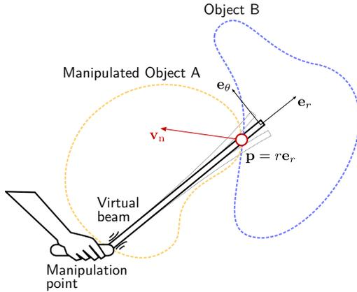
Figure 1: Description of impact and virtual beam metaphor (the handle of the haptic device is attached to Object A at the manipulation point).
