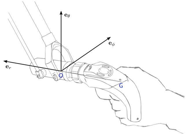
Figure 5: The three directions of torque vibration around  $\mathbf{e}_r$ ,  $\mathbf{e}_\theta$  and  $\mathbf{e}_\phi$ .
