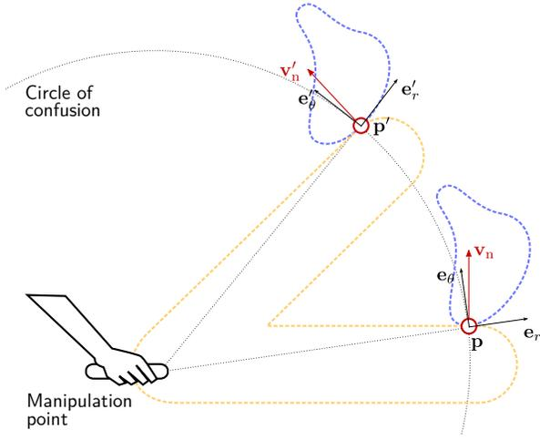
Figure 3: Circle of confusion. The two impact points  $\mathbf{p}$  and  $\mathbf{p}'$  generate the same vibration torque  $\tau(r, t)$ .
