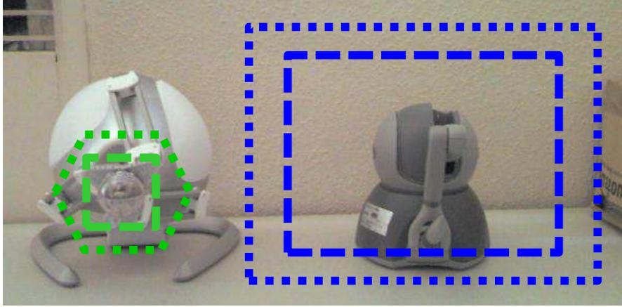
**Fig. 2** Approximate *bubble* and physical workspace sizes of a Novint Falcon and a PHANToM Omni. Inner rectangles represent the *bubbles*, while outer polygons represent the physical workspaces.
