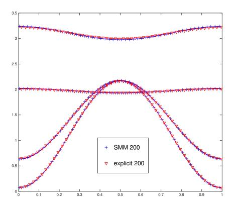
Figure 3: one-group transport equation  $\varepsilon = 1$ : summary of the previous comparisons between SMM and explicit schemes (200 grid points): Results at times t = 0.1, 0.3, 0.6 and 1 (from down to up).
