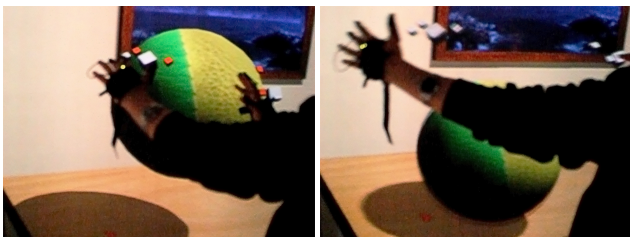
Fig. 4 User spreads her arms to release a large object without the need to further open her hands.
