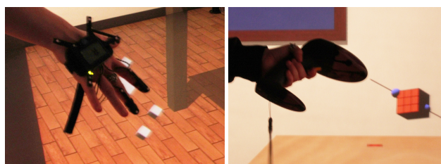
Fig. 2 Left visual representation of the palm and three fingertips in the VE (cubes are shown away from the fingers for clarity of illustration). Right wand selection used for comparison.
