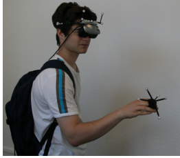
Figure 1: The Magic Barrier Tape displays the boundaries of the real workspace as a virtual barrier tape, and uses a hybrid position/rate control to travel in the scene. The user (left) “pushes” on the Magic Barrier Tape (center) to move inside the scene when he reaches the workspace boundaries. Any tracked body part can be used to trigger the Magic Barrier Tape (right).
