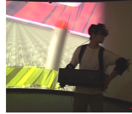
Figure 1: The Magic Barrier Tape displays the boundaries of the real workspace as a virtual barrier tape, and uses a hybrid position/rate control to travel in the scene. The user (left) “pushes” on the Magic Barrier Tape (center) to move inside the scene when he reaches the workspace boundaries. Any tracked body part can be used to trigger the Magic Barrier Tape (right).
