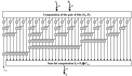
Figure 9. A 40 bit sklansky adder structure
