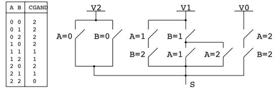
**Figure 5. The switch diagram of CGAND**
