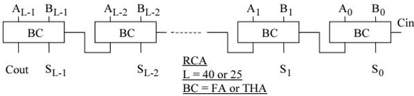
Figure 8. Synoptic diagrams of 40 bits and 25 terters RCA structures
