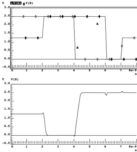
Figure 7. The CGAND simulation results
