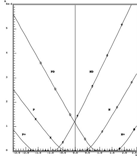
Figure 1.  $I_d(V_{gs})$  characteristics of the MOS-FETs
