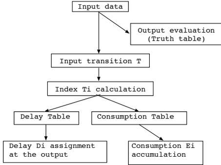
**Figure 3. Synoptic diagram of the behavioral description of a cell.**
