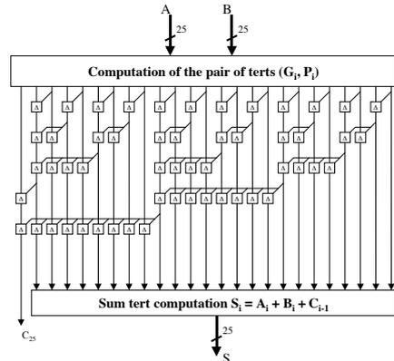
Figure 10. A 25 tert sklansky adder structure
