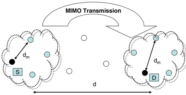
Fig. 1. Cooperative MIMO scheme for wireless sensor networks
