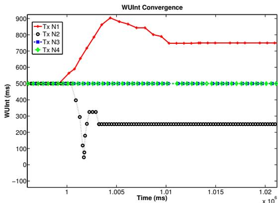
Fig. 6. Convergence of wake-up interval towards a steady state value for variable sensing rates.
