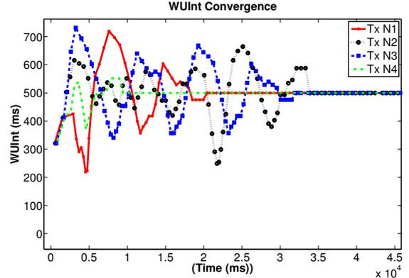
Fig. 5. Receive node adaptation with respect to transmit nodes based on the wake-up interval for a fixed data rate i.e. 1s. It is to mention here that the reference clock increment is 1 (ms), therefore all the time values are in ms.
