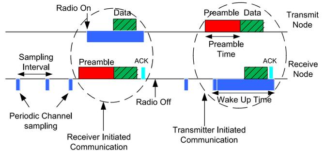
Fig. 1. General mechanism of preamble sampling protocols.
