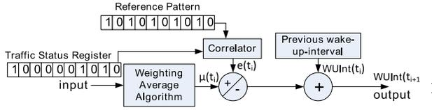
Fig. 4. Adaptive system for wake-up interval algorithm.
