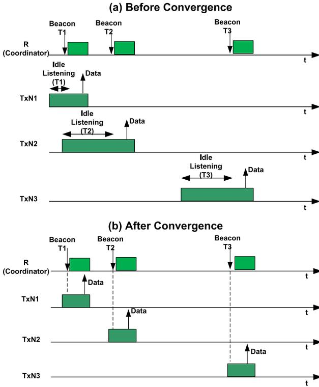
Fig. 2. Energy-latency optimized MAC protocol is divided into two phases; the evolution phase which is before convergence (a) and steady state phase which is after convergence (b).
