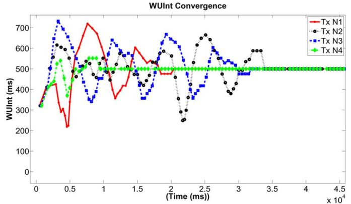
Fig. 7. Receive node adaptation with respect to transmit nodes based on the wake-up interval for a fixed data rate i.e., 1 s. It is to mention here that the reference clock's increment is 1 (ms), therefore all the time values are in ms.
