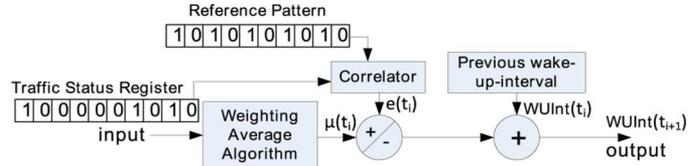
Fig. 6. Adaptive wake up interval algorithm.
