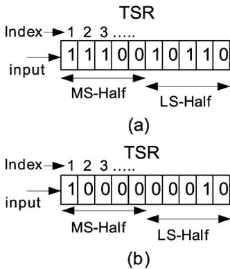
Fig. 5. Different TSR patterns are possible in the register depending upon the variations in traffic and position of the nodes.
