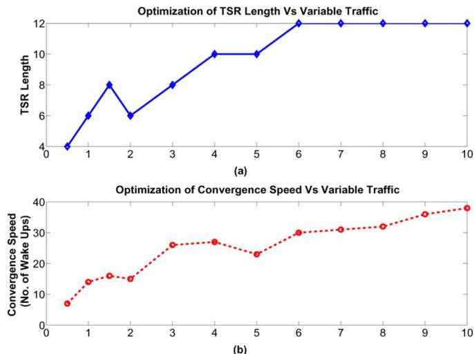
Fig. 9. Zoomed version of Fig. 8 to show convergence after changing the traffic rate. It can be seen that the receive node converges very fast as the appropriate TSR length is selected based on the indication from the packet type. The traffic rate for node 1 and node 2 changes from 1 to 1.5 s and 500 ms, respectively. Node 1 converges to a steady wake-up interval value of 750 ms, whereas node 2 converges to 250 ms for the traffic pattern of [10101010...].
