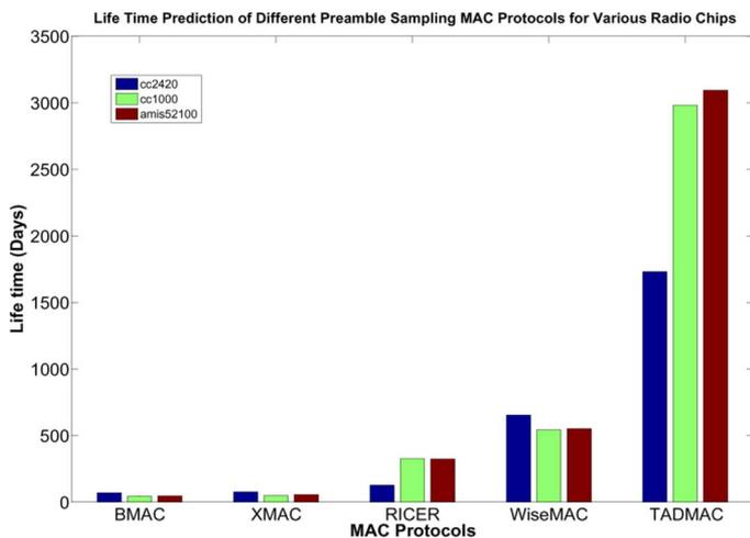
Fig. 12. Lifetime prediction of AA alkaline battery is evaluated for various MAC protocols and radio chips. TAD-MAC along with *amis52100* or *cc1000* radio chips have major difference in comparison with other MAC protocols and *cc2420*. It is noteworthy to mention here that for low traffic rate *amis52100* and *cc1000* are preferable but for higher traffic rate *cc2420* is more suitable.
