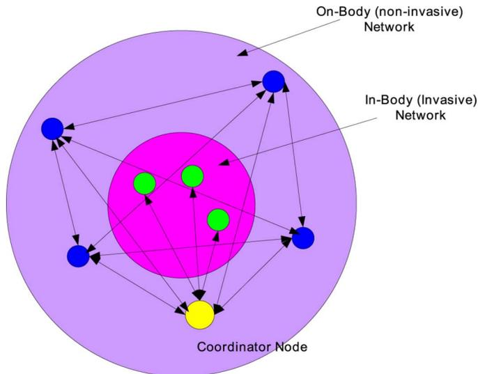
Fig. 2. Hybrid network topology: invasive sensor nodes are connected with a coordinator through star network, whereas, noninvasive nodes are configured through mesh topology.
