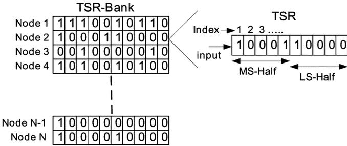
Fig. 4. Traffic shift register bank: it contains  $N$  registers for  $N$  neighbor nodes. If the receive node receives data the register (of that specific node) is filled with '1' and if it does not receive data TSR filled with '0'. The new data (either 1 or 0) is filled in the first index of the register. The register contents are shifted one bit right before inserting a new data.
