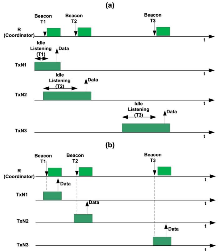
Fig. 3. Traffic-aware dynamic MAC protocol is divided into two phases: (a) the evolution phase which is before convergence and (b) steady state phase which is after convergence. It is important to note that in the second phase the receive node (coordinator) has adapted its WUInt schedule as such that the idle listening is minimized.
