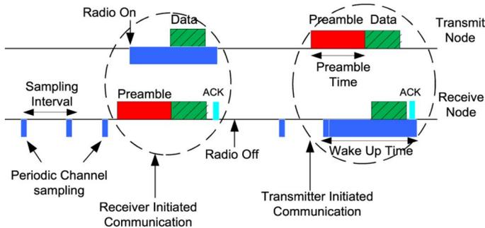
Fig. 1. General mechanism of preamble sampling protocols. Communication can either be initiated by receive or transmit node.
