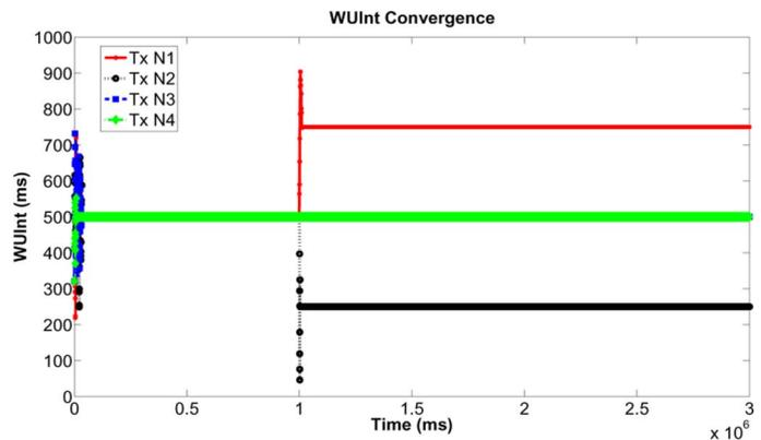
Fig. 8. Convergence of wake-up interval towards a steady state value for variable sensing rates. The traffic rate for node 1 and node 2 changes from 1 to 1.5 s and 500 ms, respectively.
