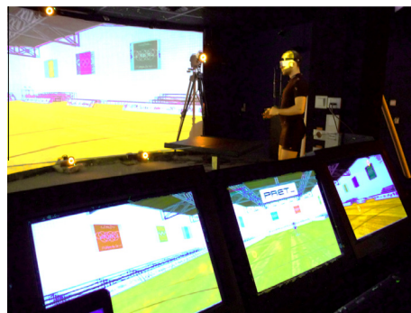
Fig. 3. The VR center composed of a control station, three video projectors (not visible on the figure above), a semicylindrical screen and stereoscopic glasses.
