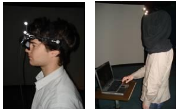
Figure 1: The experimental apparatus. Left: the participant wearing the HMD and the tracking equipment. Right: the participant equipped and wearing the opaque fabric in front of the table with the laptop computer.
