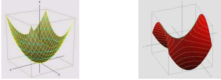
Figure 6: For d = 2 , two typical shapes quadratic forms. The bowl (left) when all eigenvalues of A are positive, and the saddle (right) when eigenvalues of A have opposite signs.
