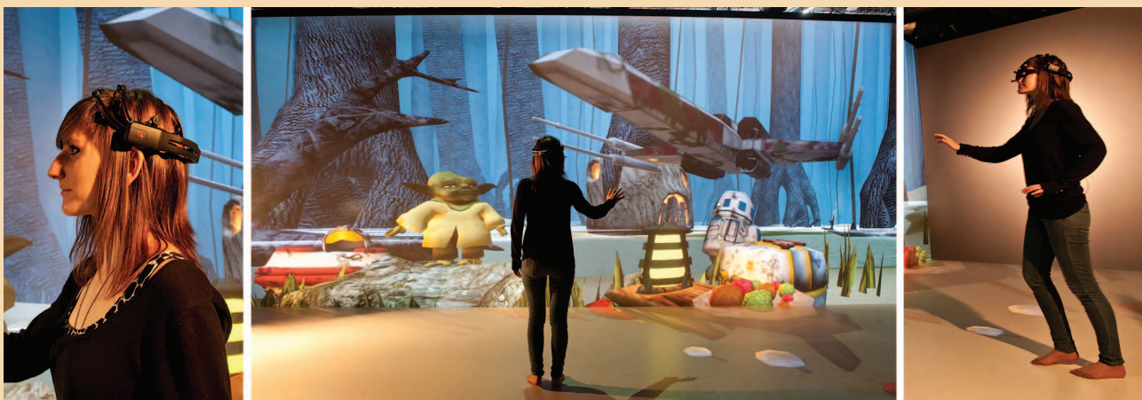
Figure B. Entertaining mind-based interaction in an immersive VE inspired by a scene in Star Wars: The Empire Strikes Back . To “lift” virtual objects, such as a helmet or a virtual spaceship partially immersed in muddy water, users simply concentrated or relaxed, depending on the playing mode.
