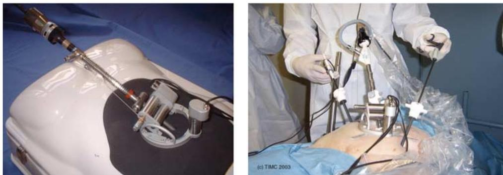
**Fig. 2.** The Light Endoscopic Robot (TIMC, Grenoble Hospital and School of Medicine): on a phantom (left), urological intervention on cadaver (right).
